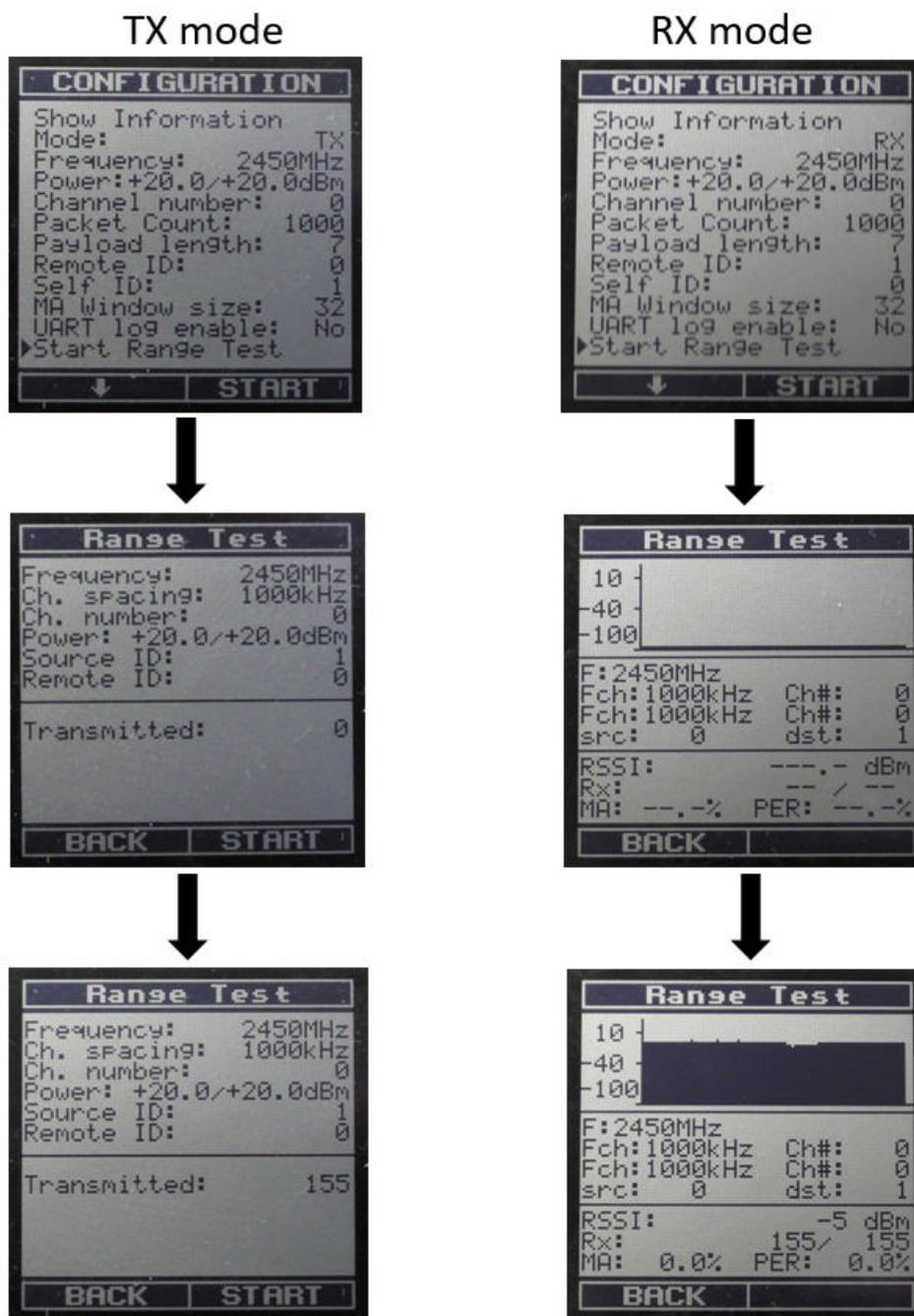
**Figure 3.3. Configure and Operate the Range Test**
